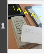
Hold the card key over the card key unit. The reverse side of the card does not matter. A short tone sounds and the rack is unlocked.
